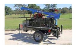
The LST1A+HD has all the features of the LST1A+ but offers enhanced power and capabilities, with increased pullback/push force and as much as 1,100 foot-pounds of torque to handle challenging soils. The machine can drill a 6-inch borehole to 100 feet at up to 100 rpm.
