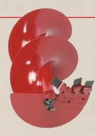
These augers feature rugged flighting, heavy-duty teeth and side cutting blades that quickly cut through tough, rocky soils. The augers can be used with 20:1 or 13:1 gear ratio transmissions and should be operated at slower RPMs than standard augers for optimal results.
