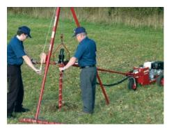
Little Beaver's hydraulic earth drill pairs with a tripod kit for the ultimate portability and value in soil sampling. Equipped with a powerful hydraulic drive and 11-horsepower engine, the hydraulic earth drill delivers excellent control and smooth sample lifting. The tripod kit is quick to set up and designed specifically for taking soil samples.
