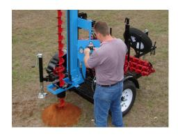
The fully hydraulic LST1A+ comes mounted on a rugged-but-lightweight single-axle trailer and features an auger head drive that makes it well-suited for drilling holes to examine soil cuttings. Its three leveling jacks allow for fast setup and stable drilling. The machine can drill a 6-inch borehole to 50 feet with a hollow stem auger or drill as deep as 100 feet with a standard auger. Then the rotary swivels aside for easy access to the borehole.
